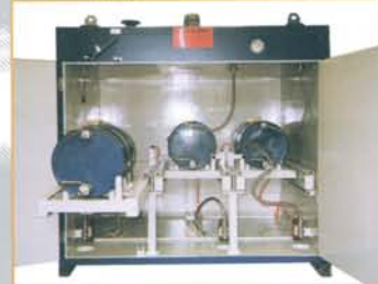
Steam heating cabinet with loading platform (Vitamins)
